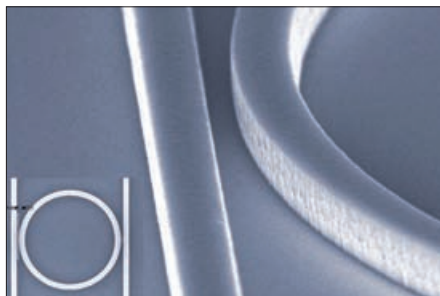
Up close: the coupling region of a micro-ring resonator using silicon-on-insulator technology, as fabricated by AMO GmbH.
